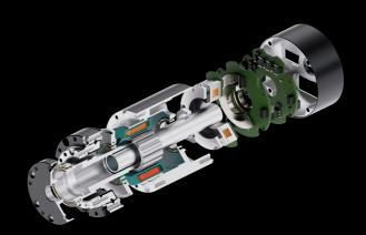
With hollow-shaft, harmonic reducer, dual encoders, magnetic brake, and brushless motorization, they deliver longlife reliability, effortless integration, and the assurance of Niryo's complete technology expertise.
